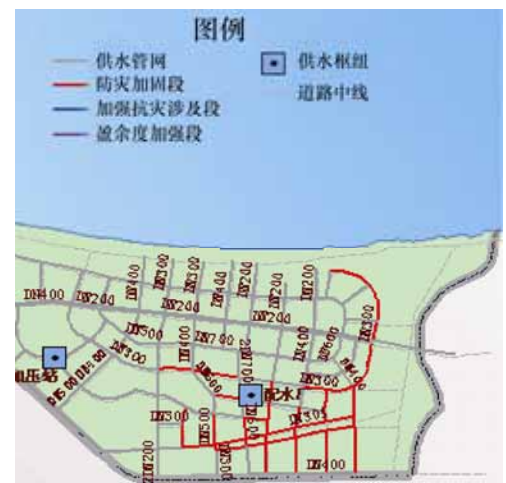
图 2 给水管网综合防灾规划的局部图 Fig. 2 Local map of W\water supply pipeline comprehensive disaster prevention plan
