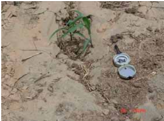
图 8 青川县板桥镇震时出现地裂缝及喷砂现象 Fig. 8 Ground fissure and sand spouts during Wenchuan earthquake in Banqiao town, Qingchuan county
